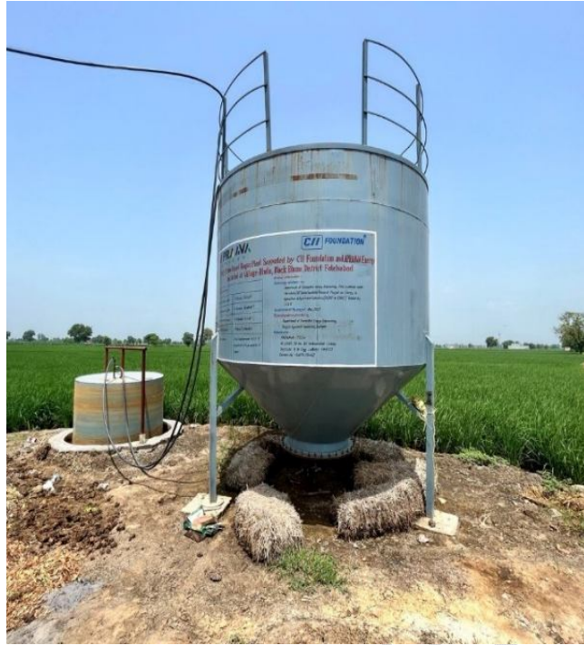
Fig. 2: PAU Model Batch Type Paddy Straw Biogas Plant at Dholu village
