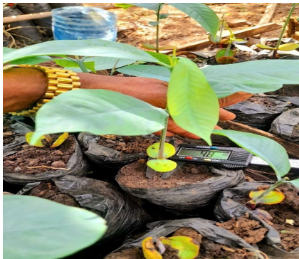
Figure9: Measuring the Diameter at the collar of an Irvingia gabonensis seedling using a caliper
