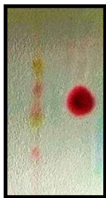
Figure 1. TLC plate showing spots having different Rf values (0.79, 0.71, 0.63, 0.59 & 0.31) of methanolic extract of A. marmelousleaves
