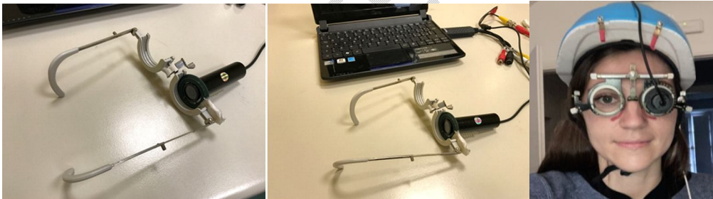
Fig. 3. The acquisition system, made of a small infrared camera mounted on a frame lens aiming at the eye not under examination and connected to a second screen placed in front of the operator.
