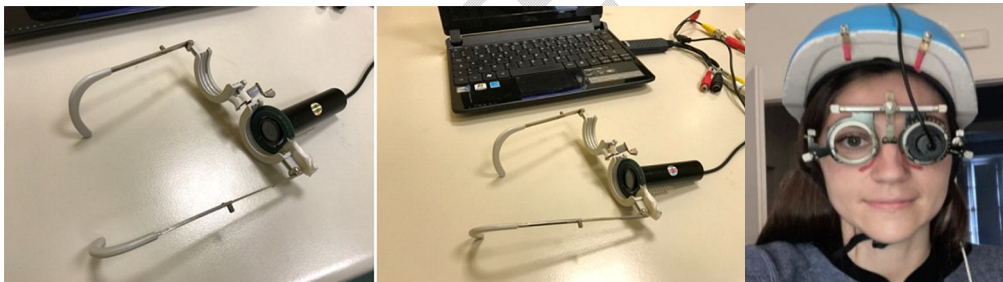
Fig. 3. The acquisition system was made of a small infrared camera mounted on a frame lens aiming at the eye not under examination and connected to a second screen placed in front of the operator.
