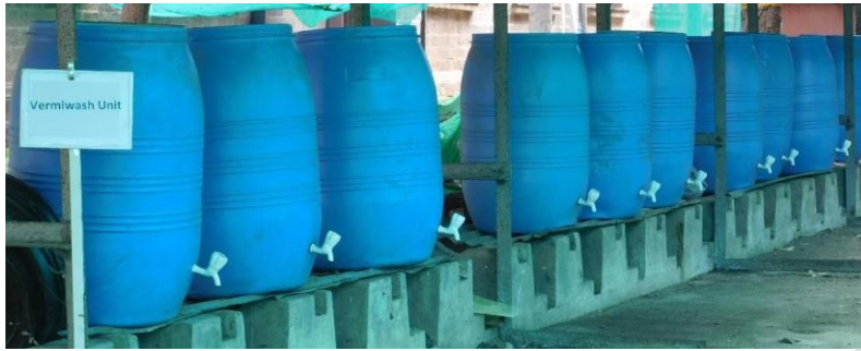
Figure 3 Vermivash unit with 200-liter plastic drums
