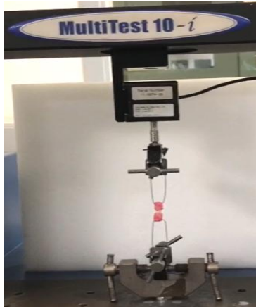
Fig 13: Sample subjected to Microshear stress
