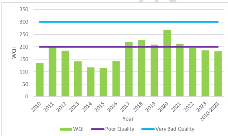
Figure 3 Water Quality Index (WQI) of Lake Chapala by year and over the entire period 2010-2023
