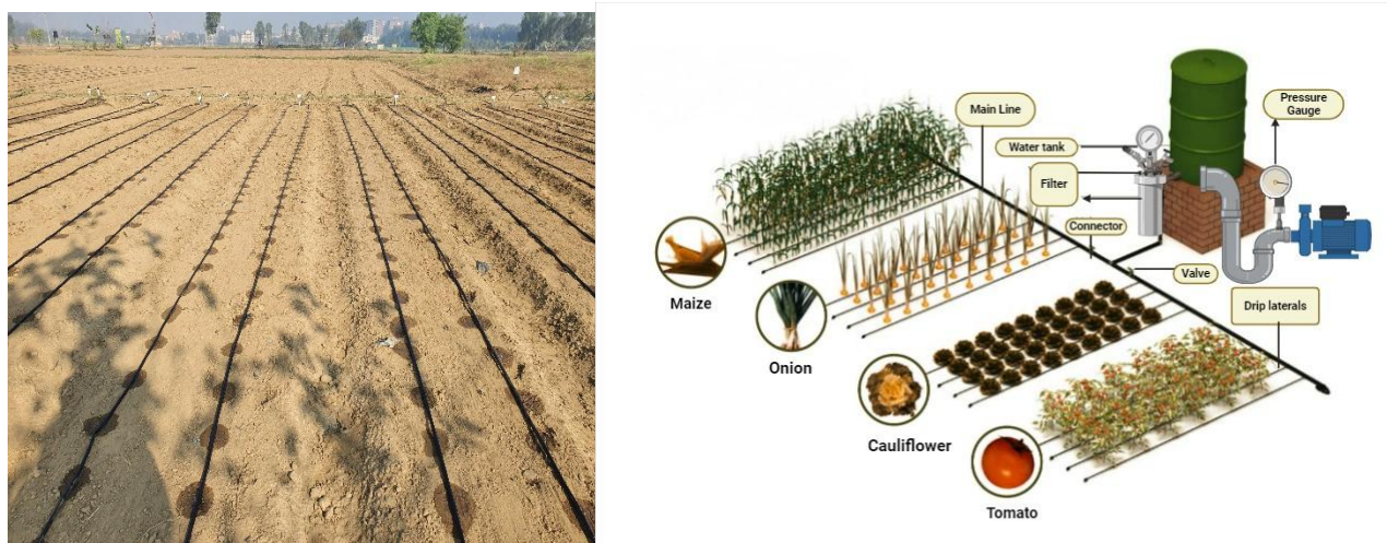
Figure 3. Layout of a complete drip irrigation system
