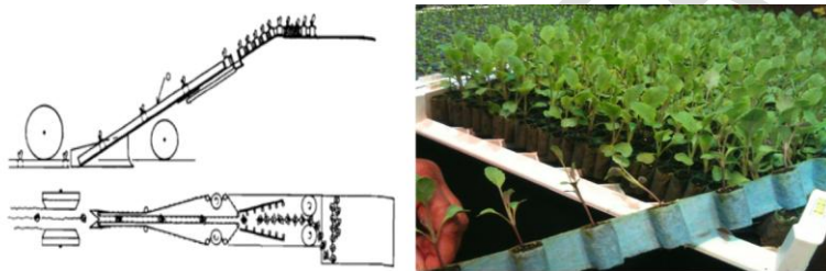
Figure 5: Schematic of Plant Tape Transplanter and Plant tape
