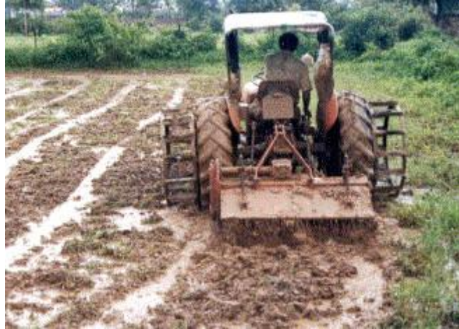
Fig.1 : Puddling on a Wetland (Verma and Dewangan, 2006)
