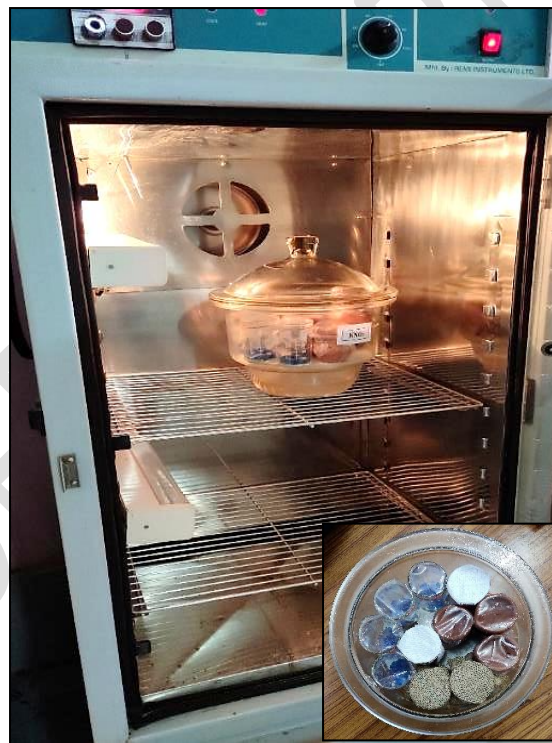
108 109 110 111 112 113 114 115 116 117 118 119 120 121 122 123 124 125 126 127 128 129 130 131 Fig. 2. Experimental setup for determination of water vapour permeability of packaging materials
