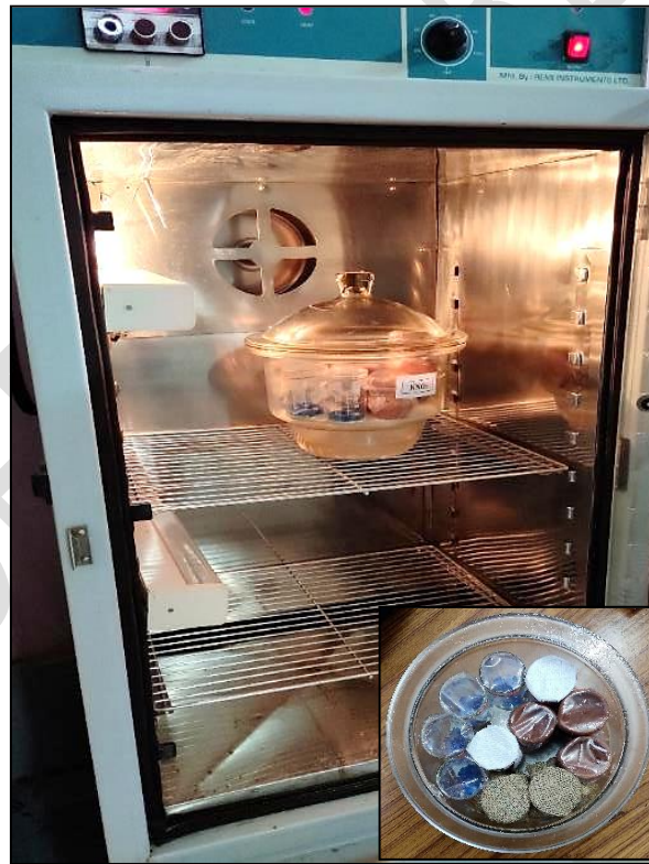
Fig. 2. Experimental setup for determination of water vapor permeability of packaging materials
