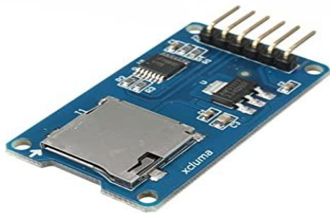
Figure 3: Data Logger Module
