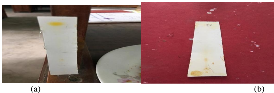
Figure 6: TLC plates of carotene developed in benzene solution (a), and iodine chamber (b)
