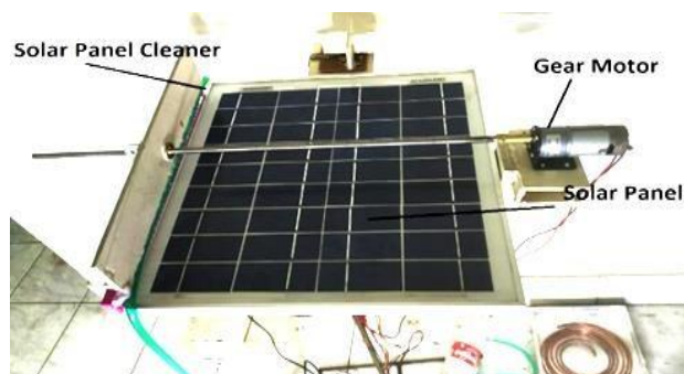
232 233 234 Fig. 11. Top view of solar sun tracking and cleaning system.
