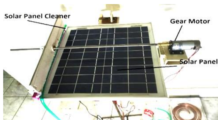
Fig. 11. Top view of solar sun tracking and cleaning system.
