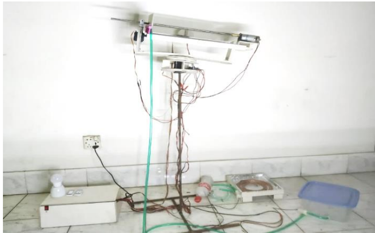
223 Fig. 10. Implemented dual-axis solar tracking, panel cleaning, and power management 224 system project.
