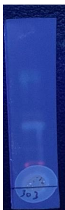
Figure 2: TLC Visualization of GandhagaThailam at 366 nm
