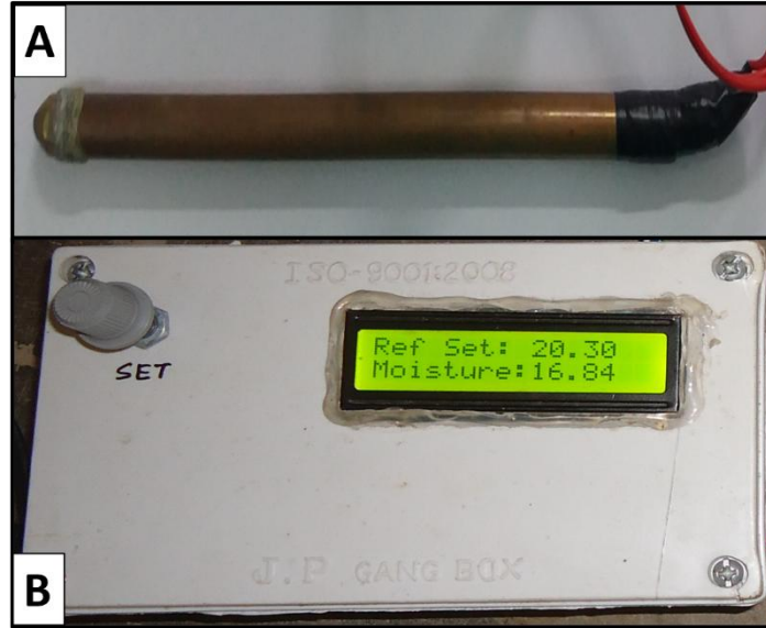
Fig.1: (A) Developed soil moisture sensor (sensing unit) (B) Controller and display units
