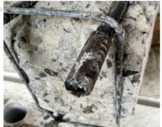
Fig. 13. (a) Failure location of steel rebar (b) Detail failure condition of steel rebar.
