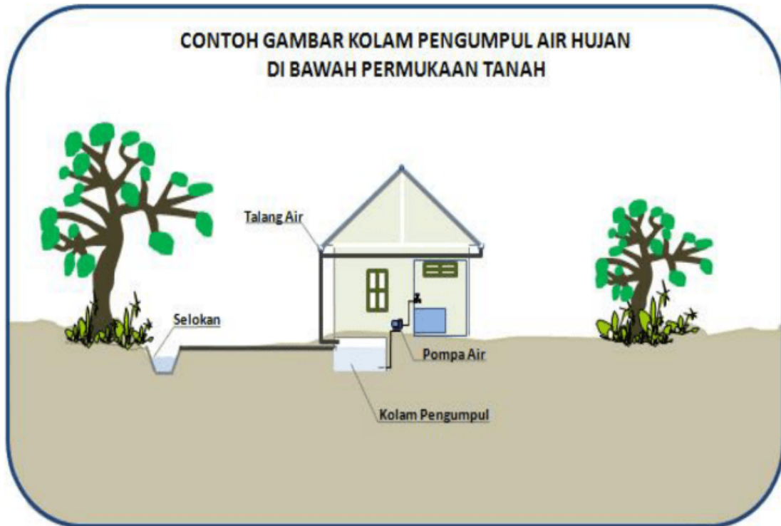
Figure 4. Rainwater Collection Pond 1
