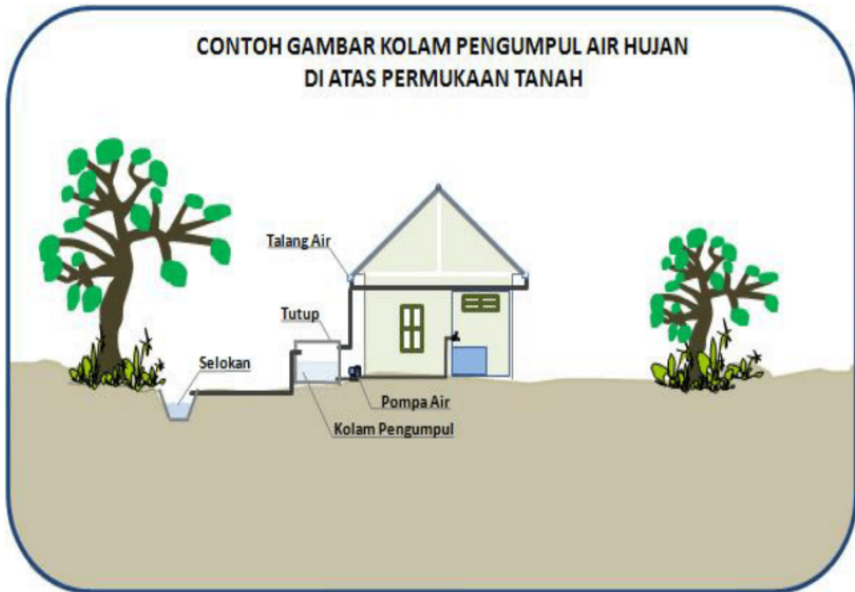
Figure 5. Rainwater Collection Pond 2
