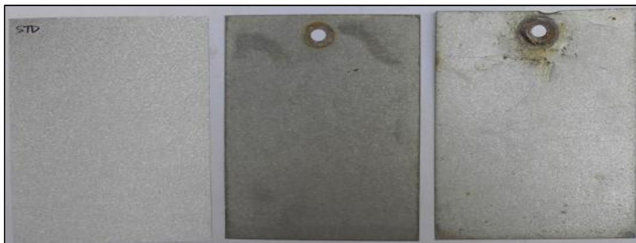
Figure 5: A photograph showing comparison of corroded specimen (AZ 150) at Mariakani and Diani test sites A control specimen, (B) -Mariakani specimen, and (C) - Diani site specimen).
