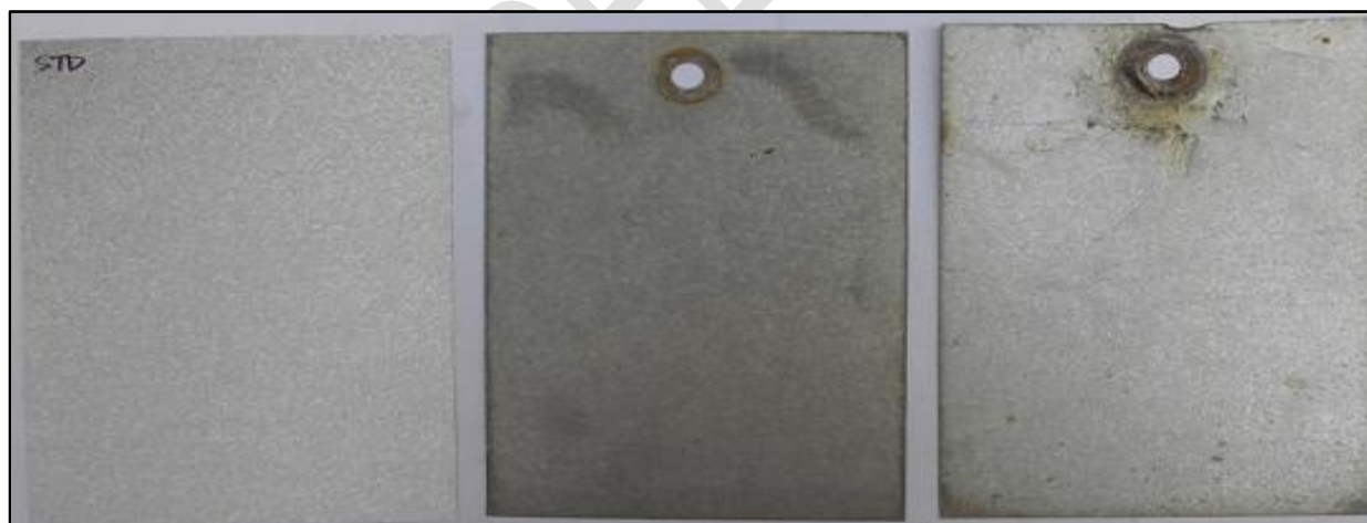
Figure 5: A photograph showing comparison of corroded specimen (AZ 150) at Mariakani and Diani test sites (S1-control specimen, S2- Mariakani specimen and S3- Diani site specimen).
