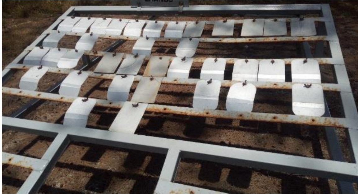
Figure 2: A set-up for outdoor exposure of 55% Al-Zn metallic coated sheets at Diani site.
