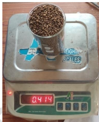
Fig.3. Measurement the bulk density for granular fertilizers
