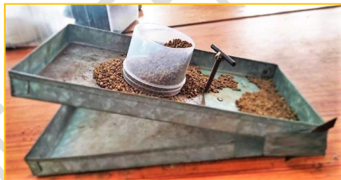
Fig.4. Measurement the coefficient of friction for granular fertilizers
