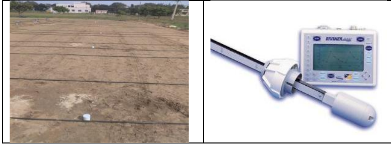
Plate 2 Installed access tubes and FDR sensor
