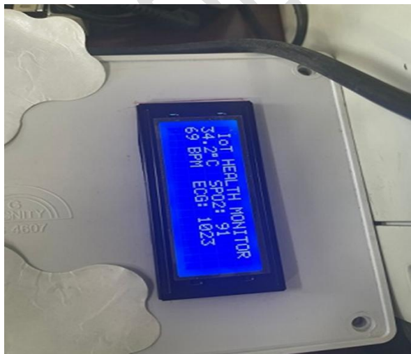
Figure4: Testing to acquire values for ECG, Body temperature and SPO2 Measurement
