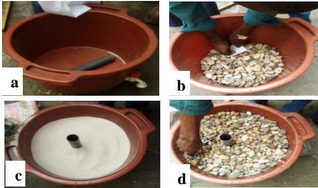
Figure 3 : Experimental device assembly (a): PVC tank and distribution pipe; (b) : filling of coarse gravel; (c) : filling of sand and aeration pipe; (d) filling of fine gravel also called control filter (T-F)
