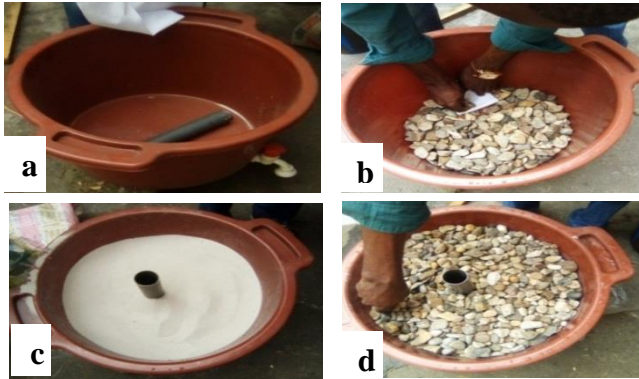
Figure 3 : Experimental device assembly (a): PVC tank and distribution pipe; (b) : filling of coarse gravel; (c) : filling of sand and aeration pipe; (d) filling of fine gravel also called control filter (T-F)
