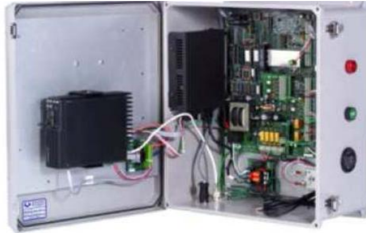
Figure 4. Automation Electronics AEPOC 2100 controller
