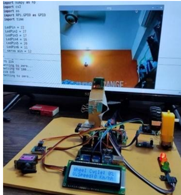
Fig. 11. The face and eyes are not detected, the Red LED is on, Yellow and Green LEDs are off. The wheel motor is not rotating, and the servo motor is at 180°.
