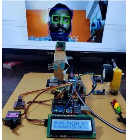
Fig.9. The face and eyes of the driver are detected, the Yellow LED and Green LED are on, the Red LED is off. The wheel motor is rotating, and the servo motor is at 90°.
