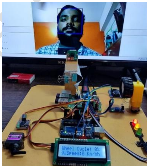
Fig. 10. The face of the driver is detected but the eyes are not detected. The Yellow and Red LEDs are on, and the Green LED is off. The wheel motor is not rotating, and the servo motor is at 180°.
