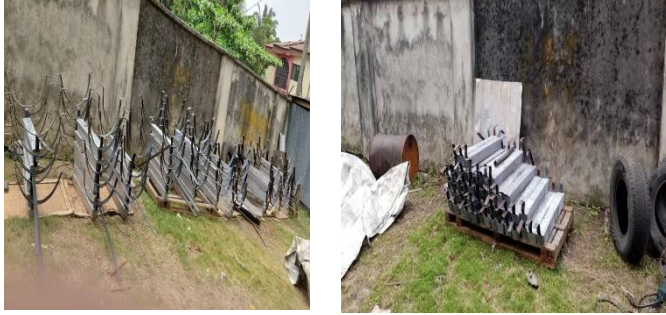
Fig. 2. Images of the fabrication of the anode-clamp assembly
