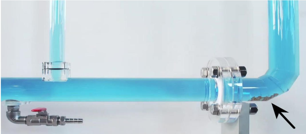
Fig.4. The pieces of glass stop at the elbow of the vertical pipe
