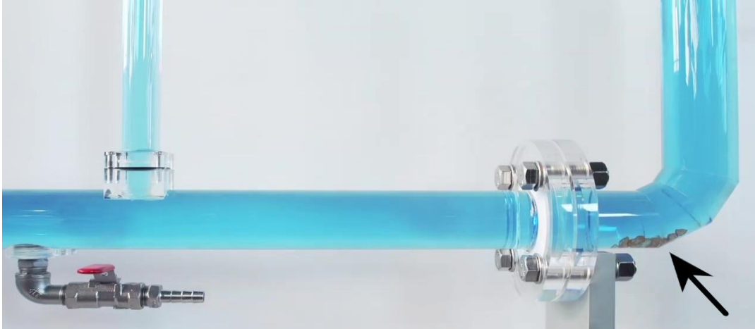
Fig.5. The pieces of glass stop at the elbow of the vertical pipe
