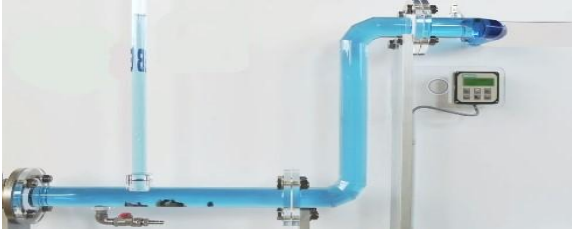
Fig.2. Transport pipe made of transparent acrylic resin
