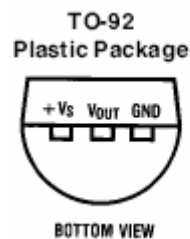
Figure 1: Bottom view of LM35 temperature sensor showing pin out
