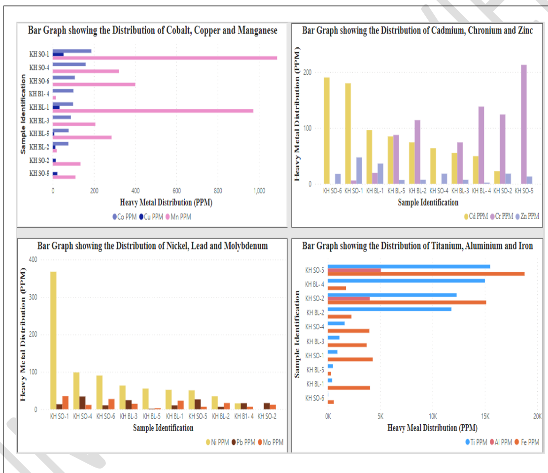
Figure 4. Graphs showing the mean distribution of each heavy metal at the sample locations for the Study Areas. Samples retrieved from the Tailings Pond show higher values compared to samples retrieved from Blue Lake.
