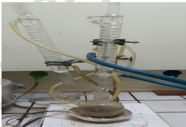
Fig. 1 Reflux system for phthaloylation reaction of chitosan
