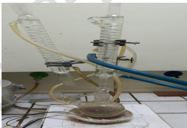
Fig. 1 Reflux system for phthaloylation reaction of chitosan
