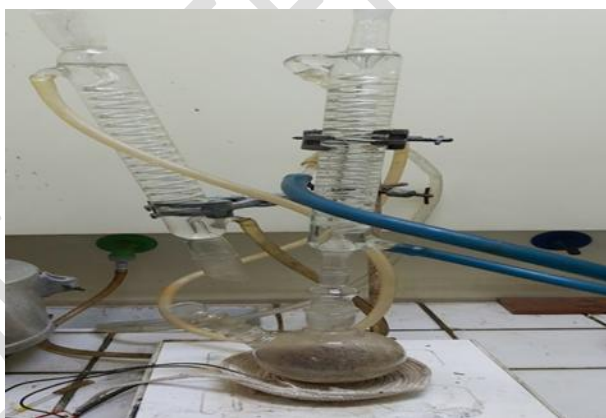
Fig. 1 Reflux system for phthaloylation reaction of chitosan
