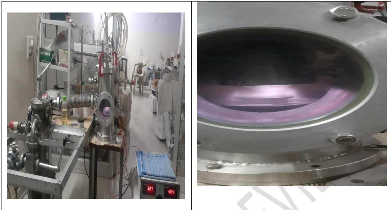
Fig.1 A. plasma discharge treatment chamber (left) B. mustard seeds undergoing in a plasma reactor (right)
