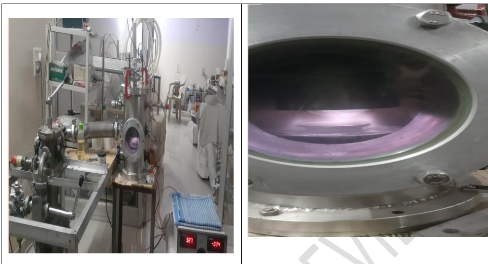
Fig.1 A. plasma discharge treatment chamber B. mustard seeds undergoing in plasma reactor
