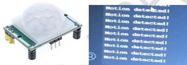
Fig.12 PIR Motion Sensor with its readings
