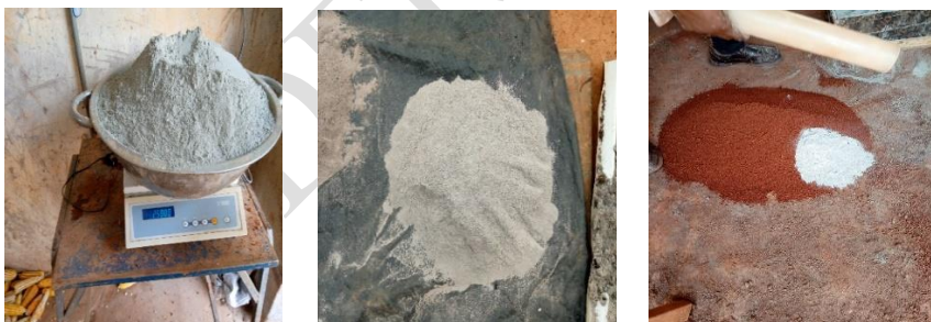
Figure 7: Batching of the various aggregates in percentages.
