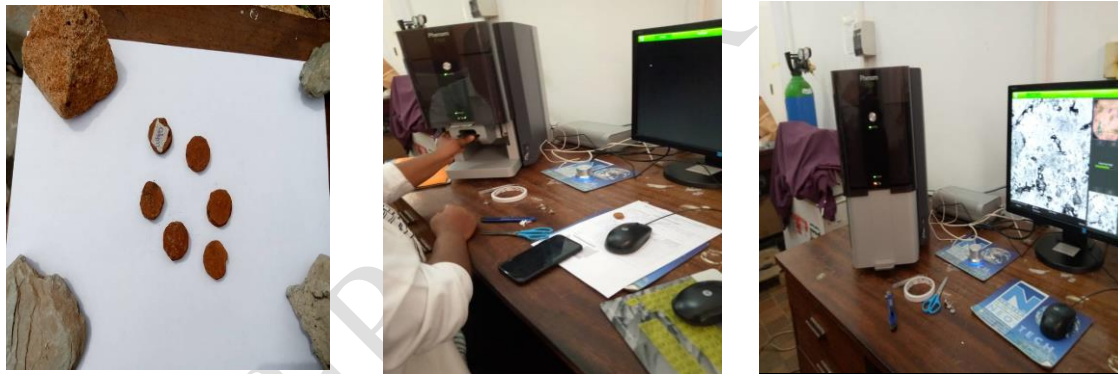
Figure 3 & 2: EDS and SEM analysis of compressed laterite interlocking blocks set up
