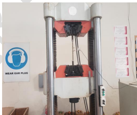
Figure 2: Tensile test setup.
