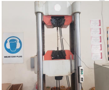
Figure 2: Tensile test setup.
