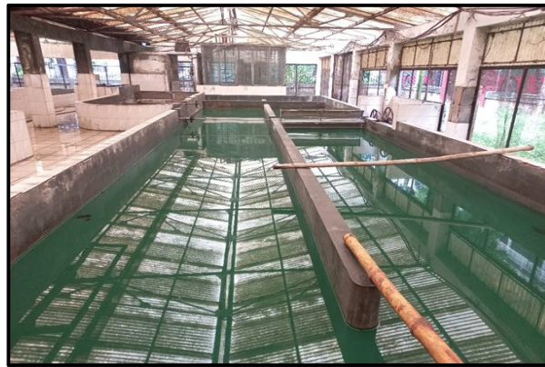
101 Fig. 2. Spirulina platensis raceway pond at BCSIR Laboratories, Dhaka
