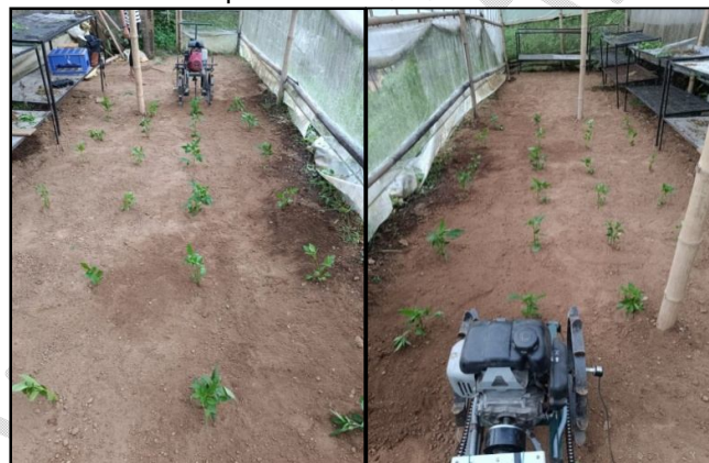
(a) Front view of weeder (b) Back view of weeder
